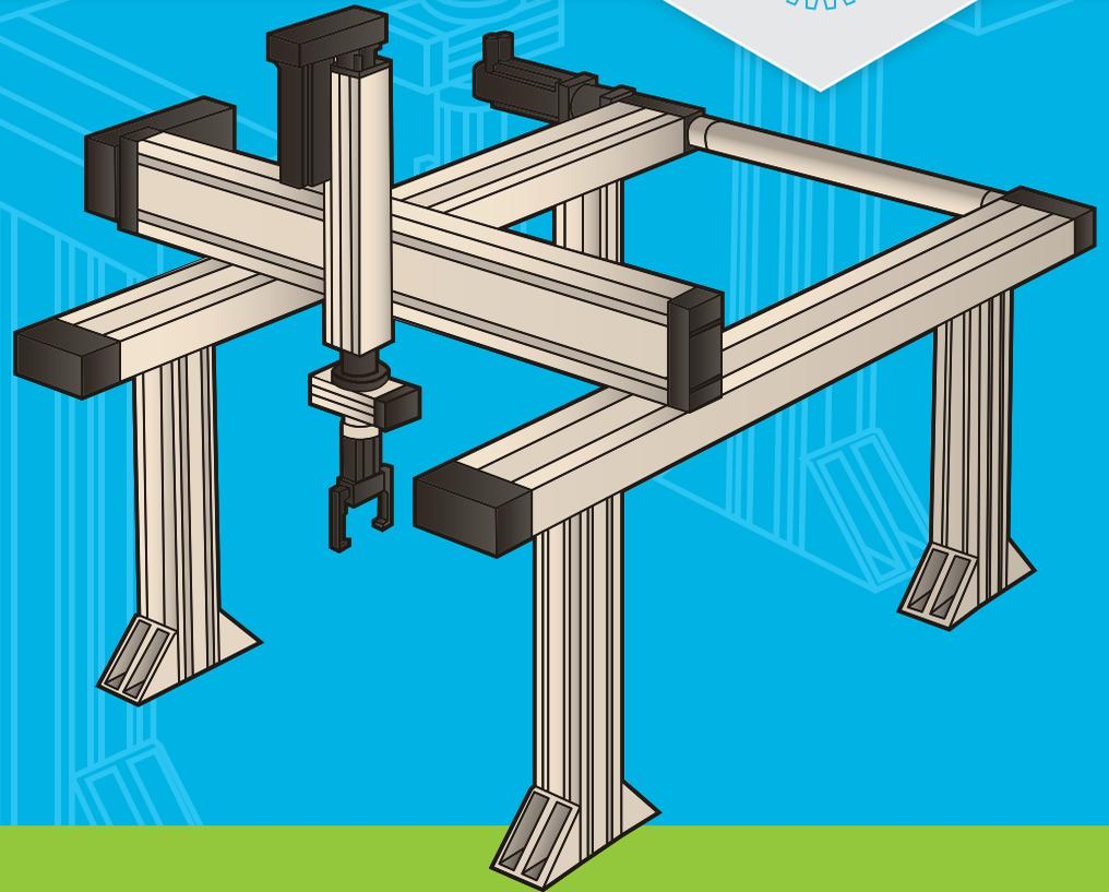
Cartesian robots typically consist of 2-3 linear actuators assembled to fit a particular application. By their nature, Cartesian robots are positioned above the intended workspace and can be elevated above to maximize available floor space and accommodate a wide range of workpiece sizes. When placed on an elevated structure suspended
