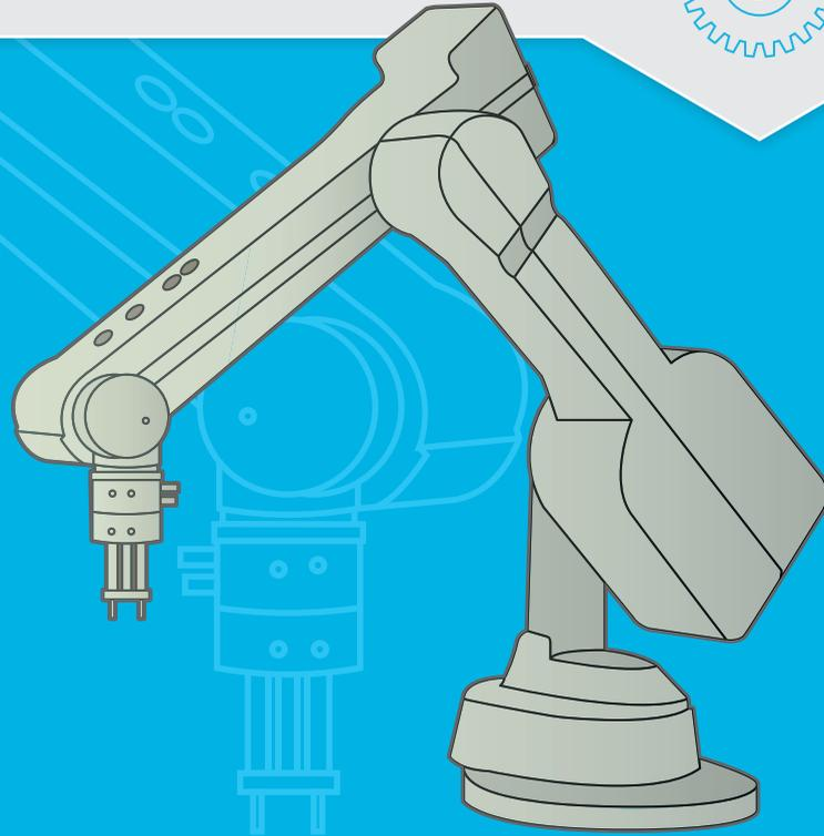
An articulated robot is the type of robot that comes to mind for most people. Similar to a human arm, an articulated robot is classified by the number of points of rotation or axes (joints) such as the most common, the 6-axis articulated robot. There are also
