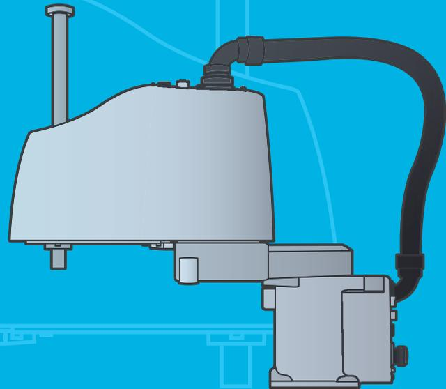
Selective Compliance Assembly (or Articulated) Robot Arm. Slightly compliant in X-Y, horizontal, plane, but rigid in Z (vertical) direction. Generally a 4-axis unit, with most under 13lb (6kg) payload capacity and 25" (650mm) of reach.
